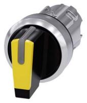
Selector switch, illuminable, 22 mm, round, metal, shiny, yellow, selector switch, short, 3 switch positions I>O<II, momentary contact type, actuating angle  $2x45^{\circ}$ , 10:30h/12h/13:30h, Z=50-unit packaging
