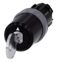
key-operated switch Siemens, 22 mm, round, plastic with metal front ring, lock number SSG10, with 2 keys, 3 switch positions I>O<II, momentary contact on the left, latching on the right, actuating angle 2x45°, 10:30h/12h/13:30h, key removal O+II, with laser labeling, upper case and lower case, always upper case at beginning of line
