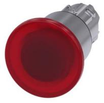
Illuminated mushroom pushbutton, 22 mm, round, metal, shiny, red, 40 mm, 3 switch positions, latches after pushing in, unlatches by pull-to-unlatch mechanism to center position, after pulling out the button Retraction to center position, Z=50-unit packaging
