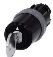
key-operated switch Siemens, 22 mm, round, plastic with metal front ring, special lock, with 2 keys, 3 switch positions I>O<II, momentary contact type, actuating angle  $2x45^{\circ}$ , 10:30h/12h/13:30h, key removal O
