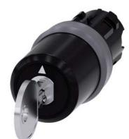
key-operated switch Siemens, 22 mm, round, plastic with metal front ring, lock number SSG10, with 2 keys, 3 switch positions I-O-II, latching, actuating angle 2x45°, 10:30h/12h/13:30h, key removal I, with laser labeling, lower case
