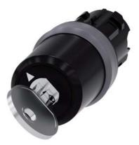
key-operated switch Siemens, 22 mm, round, plastic with metal front ring, lock number SSG10, with 2 keys, 2 switch positions O<1, momentary contact type, actuating angle 45°, 10:30h/12h, key removal O, with laser labeling, upper case and lower case, always upper case at the beginning of the word
