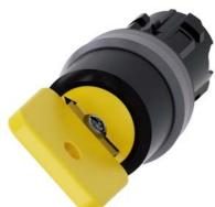
Key-operated switch O.M.R, 22 mm, round, plastic with metal front ring, lock number 73033, yellow, with 2 keys, 2 switch positions O-I, latching, actuating angle 90°, 10:30h/13:30h, key removal O+I, with laser labeling, upper case and lower case, always upper case at beginning of line
