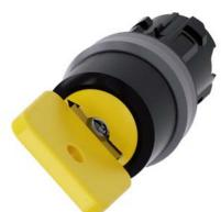
Key-operated switch O.M.R, 22 mm, round, plastic with metal front ring, lock number 73033, yellow, with 2 keys, 2 switch positions O-I, latching, actuating angle 90°, 10:30h/13:30h, key removal O, with laser labeling, inscription or symbol Customer-specific selection with SIRIUS ACT configurator (CIN)
