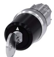
Key-operated switch BKS, 22 mm, round, metal, shiny, lock number S1, with 2 keys, 3 switch positions I>O<II, momentary contact on the left, latching on the right, actuating angle 2x45°, 10:30h/12h/13:30h, key removal O, with laser labeling, inscription or symbol Customer-specific selection with SIRIUS ACT configurator (CIN)
