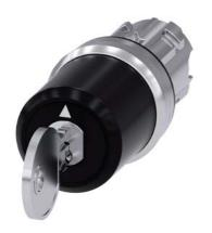
Key-operated switch BKS, 22 mm, round, metal, shiny, lock number S1, with 2 keys, 3 switch positions I-O<II, left latching, right momentary contact type, actuating angle 2x45°, 10:30h/12h/13:30h, key removal O+I, with laser labeling, inscription or symbol Customer-specific selection with SIRIUS ACT configurator (CIN)
