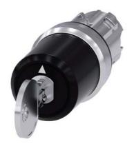
Key-operated switch BKS, 22 mm, round, metal, shiny, lock number S1, with 2 keys, 3 switch positions I-O-II, latching, actuating angle 2x45°, 10:30h/12h/13:30h, Key removal I+O+II, with laser labeling, upper case
