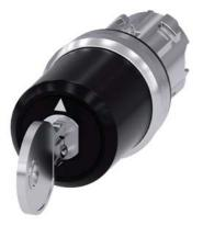
Key-operated switch BKS, 22 mm, round, metal, shiny, lock number S1, with 2 keys, 3 switch positions I-O-II, latching, actuating angle 2x45°, 10:30h/12h/13:30h, key removal O, Z=50-unit packaging
