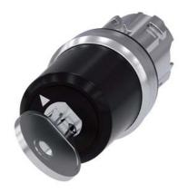
Key-operated switch BKS, 22 mm, round, metal, shiny, lock number S1, with 2 keys, 2 switch positions O-I, latching, actuating angle 90°, 10:30h/13:30h, key removal O, Z=50-unit packaging
