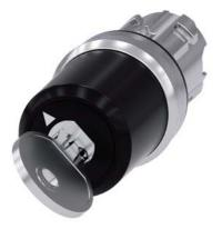
Key-operated switch BKS, 22 mm, round, metal, shiny, lock number S1, with 2 keys, 2 switch positions O<I, momentary contact type, Actuating angle  $45^\circ,$  10:30h/12h, key removal O, with laser labeling, lower case
