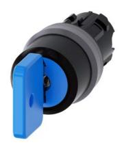
Key-operated switch O.M.R, 22 mm, round, plastic with metal front ring, lock number 73038, blue, with 2 keys, 3 switch positions I-O-II, latching, actuating angle 2x45°, 10:30h/12h/13:30h, Key removal I+O+II, with laser labeling, lower case
