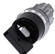
key-operated switch Siemens, 22 mm, round, metal, shiny, lock no. VL5, with 2 keys, 2 switch positions O-I, latching, actuating angle 90°, 10:30h/13:30h, key removal O, with laser labeling, upper case and lower case, always upper case at the beginning of the word
