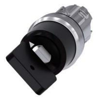
key-operated switch Siemens, 22 mm, round, metal, shiny, lock no. VL5, with 2 keys, 2 switch positions O-I, latching, actuating angle  $90^\circ$ , 10:30h/13:30h, key removal O, with laser labeling, upper case and lower case, always upper case at beginning of line
