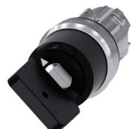
key-operated switch Siemens, 22 mm, round, metal, shiny, lock no. VL5, with 2 keys, 2 switch positions O<I, momentary contact type, actuating angle 45°, 10:30h/12h, key removal O, with laser labeling, upper case and lower case, always upper case at the beginning of the word
