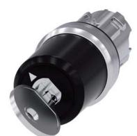
key-operated switch Siemens, 22 mm, round, metal, shiny, lock no. LSG1, with 2 keys, 2 switch positions O-I, latching, actuating angle 90°, 10:30h/13:30h, key removal O+I, with laser labeling, upper case
