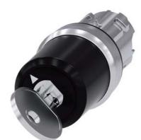
key-operated switch Siemens, 22 mm, round, metal, shiny, lock no. LSG1, with 2 keys, 2 switch positions O-I, latching, actuating angle 90°, 10:30h/13:30h, key removal O+I, with laser labeling, upper case and lower case, always upper case at beginning of line
