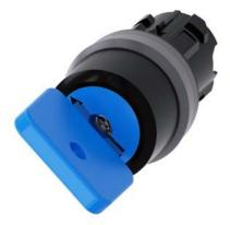
Key-operated switch O.M.R, 22 mm, round, plastic with metal front ring, lock number 73038, blue, with 2 keys, 2 switch positions O-I, latching, actuating angle 90°, 10:30h/13:30h, key removal O+I, with laser labeling, upper case
