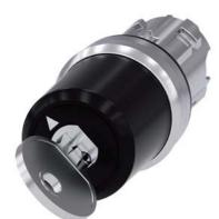
key-operated switch Siemens, 22 mm, round, metal, shiny, lock no. LSG1, with 2 keys, 2 switch positions O-I, latching, actuating angle 90°, 10:30h/13:30h, key removal O, with laser labeling, upper case and lower case, always upper case at the beginning of the word
