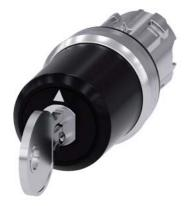
key-operated switch Siemens, 22 mm, round, metal, shiny, lock number SSG10, with 2 keys, 3 switch positions I>O<II, momentary contact on the left, latching on the right, actuating angle 2x45°, 10:30h/12h/13:30h, key removal O+II, with laser labeling, inscription or symbol customer-specific selection with SIRIUS ACT configurator (CIN)
