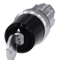
key-operated switch Siemens, 22 mm, round, metal, shiny, lock number SSG10, with 2 keys, 3 switch positions I>O<II, momentary contact on the left, latching on the right, actuating angle 2x45°, 10:30h/12h/13:30h, key removal O+II, with laser labeling, upper case and lower case, always upper case at beginning of line
