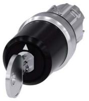
key-operated switch Siemens, 22 mm, round, metal, shiny, lock number SSG10, with 2 keys, 3 switch positions I>O<II, momentary contact on the left, latching on the right, actuating angle 2x45°, 10:30h/12h/13:30h, key removal II, with laser labeling, upper case and lower case, always upper case at the beginning of the word
