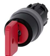
Key-operated switch O.M.R, 22 mm, round, plastic with metal front ring, lock number 73037, red, with 2 keys, 3 switch positions |O<|I|, momentary contact type, actuating angle 2x45°, 10:30h/12h/13:30h, key removal O, with laser labeling, upper case and lower case, always upper case at beginning of line
