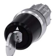
key-operated switch Siemens, 22 mm, round, metal, shiny, special lock, with 2 keys, 3 switch positions I-O<II, left latching, momentary contact type on the right, actuating angle 2x45°, 10:30h/12h/13:30h, key removal I
