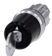
key-operated switch Siemens, 22 mm, round, metal, shiny, lock number SSG10, with 2 keys, 3 switch positions I-O<II, left latching, momentary contact type on the right, actuating angle  $2x45^{\circ}$ , 10:30h/12h/13:30h, key removal O, with laser labeling, upper case and lower case, always upper case at beginning of line
