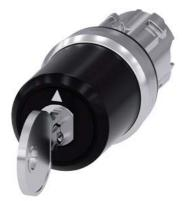
key-operated switch Siemens, 22 mm, round, metal, shiny, lock number SSG10, with 2 keys, 3 switch positions I>O<II, momentary contact type, actuating angle 2x45°, 10:30h/12h/13:30h, key removal O, with laser labeling, lower case
