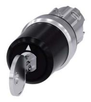
key-operated switch Siemens, 22 mm, round, metal, shiny, lock number SSG10, with 2 keys, 3 switch positions I-O-II, latching, actuating angle  $2x45^\circ$ , 10:30h/12h/13:30h, key removal I, Z=50-unit packaging
