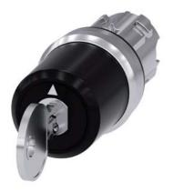
key-operated switch Siemens, 22 mm, round, metal, shiny, lock number SSG10, with 2 keys, 3 switch positions I-O-II, latching, actuating angle 2x45°, 10:30h/12h/13:30h, key removal I+O+II, with laser labeling, inscription or symbol customer-specific selection with SIRIUS ACT configurator (CIN)
