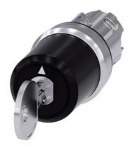
key-operated switch Siemens, 22 mm, round, metal, shiny, lock number SSG10, with 2 keys, 3 switch positions I-O-II, latching, actuating angle  $2x45^{\circ}$ , 10:30h/12h/13:30h, key removal O, Z=50-unit packaging
