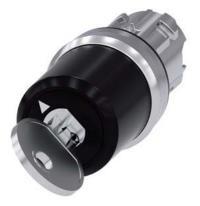
key-operated switch Siemens, 22 mm, round, metal, shiny, lock number SSG10, with 2 keys, 2 switch positions O-I, latching, actuating angle 90°, 10:30h/13:30h, key removal I, with laser labeling, upper case and lower case, always upper case at beginning of line
