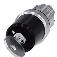
key-operated switch Siemens, 22 mm, round, metal, shiny, lock number SSG10, with 2 keys, 2 switch positions O<I, momentary contact type, actuating angle 45°, 10:30h/12h, key removal O, with laser labeling, upper case
