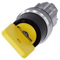
Key-operated switch O.M.R, 22 mm, round, metal, shiny, lock number 73033, yellow, with 2 keys, 2 switch positions O<I, momentary contact type, Actuating angle 45°, 10:30h/12h, key removal O, with laser labeling, upper case and lower case, always upper case at beginning of line
