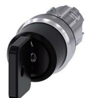
Key-operated switch O.M.R, 22 mm, round, metal, shiny, lock number 73034, black, with 2 keys, 3 switch positions I>O<II, momentary contact type, actuating angle 2x45°, 10:30h/12h/13:30h, key removal O, with laser labeling, upper case and lower case, always upper case at beginning of line
