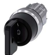
Key-operated switch O.M.R, 22 mm, round, metal, shiny, lock number 73034, black, with 2 keys, 3 switch positions I-O-II, latching, actuating angle 2x45°, 10:30h/12h/13:30h, key removal O, with laser labeling, upper case and lower case, always upper case at the beginning of the word
