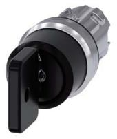
Key-operated switch O.M.R, 22 mm, round, metal, shiny, lock number 73034, black, with 2 keys, 3 switch positions I-O-II, latching, actuating angle  $2x45^{\circ}$ , 10:30h/12h/13:30h, key removal O, with laser labeling, upper case
