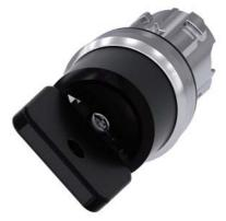
Key-operated switch O.M.R, 22 mm, round, metal, shiny, lock number 73034, black, with 2 keys, 2 switch positions O<I, momentary contact type, Actuating angle 45°, 10:30h/12h, key removal O, with laser labeling, lower case
