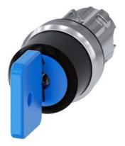
Key-operated switch O.M.R, 22 mm, round, metal, shiny, lock number 73038, blue, with 2 keys, 3 switch positions I-O-II, latching, actuating angle 2x45°, 10:30h/12h/13:30h, key removal O, with laser labeling, upper case and lower case, always upper case at the beginning of the word
