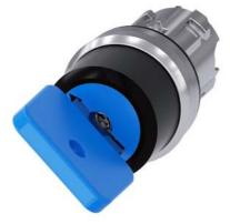
Key-operated switch O.M.R, 22 mm, round, metal, shiny, lock number 73038, blue, with 2 keys, 2 switch positions O-I, latching, actuating angle 90°, 10:30h/13:30h, key removal O+I, with laser labeling, upper case and lower case, always upper case at the beginning of the word
