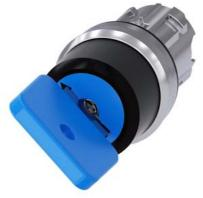
Key-operated switch O.M.R, 22 mm, round, metal, shiny, lock number 73038, blue, with 2 keys, 2 switch positions O<I, momentary contact type, Actuating angle 45°, 10:30h/12h, key removal O, with laser labeling, upper case and lower case, always upper case at beginning of line
