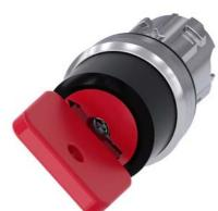
Key-operated switch O.M.R, 22 mm, round, metal, shiny, lock number 73037, red, with 2 keys, 2 switch positions O<I, momentary contact type, Actuating angle 45°, 10:30h/12h, key removal O, with laser labeling, upper case
