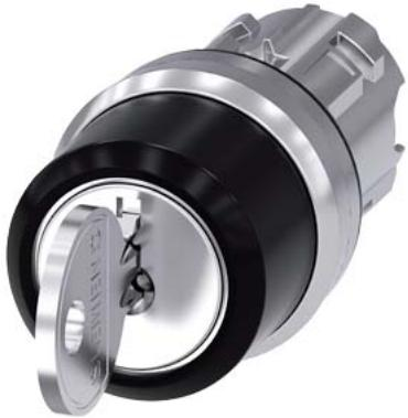
RONIS key-operated switch, 22 mm, round, metal, shiny, Lock No. 421, with 2 keys, 3 switch positions I-O-II, latching, actuating angle 2x45°, 10:30h/12h/13:30h, Key removal I+O+II, with laser labeling, upper case
