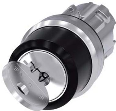
RONIS key-operated switch, 22 mm, round, metal, shiny, Lock No. 421, with 2 keys, 2 switch positions O-I, latching, actuating angle 90°, 10:30h/13:30h, key removal O+I, with laser labeling, lower case
