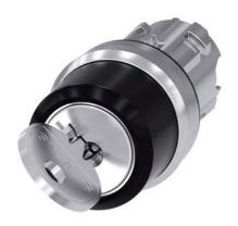
RONIS key-operated switch, 22 mm, round, metal, shiny, Lock No. 421, with 2 keys, 2 switch positions O-I, latching, actuating angle 90°, 10:30h/13:30h, key removal O+I, with laser labeling, upper case
