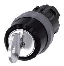
RONIS key-operated switch, 22 mm, round, plastic with metal front ring, lock number SB30, with 2 keys, 3 switch positions I-O<II, left latching, right momentary contact type, actuating angle 2x45°, 10:30h/12h/13:30h, key removal O, possible special locks: SB31, 421, 455, Z=50-unit packaging
