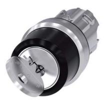
RONIS key-operated switch, 22 mm, round, metal, shiny, lock number 455, with 2 keys, 2 switch positions O-I, latching, actuating angle  $90^\circ$ , 10:30h/13:30h, key removal I, Z=50-unit packaging
