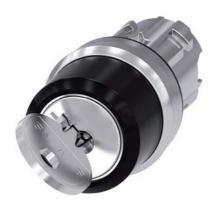
RONIS key-operated switch, 22 mm, round, metal, shiny, lock number 455, with 2 keys, 2 switch positions O-l, latching, actuating angle 90°, 10:30h/13:30h, key removal O+l, with laser labeling, inscription or symbol Customer-specific selection with SIRIUS ACT configurator (CIN)
