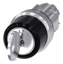
RONIS key-operated switch, 22 mm, round, metal, shiny, lock number SB30, with 2 keys, 3 switch positions I-O-II, latching, actuating angle 2x45°, 10:30h/12h/13:30h, key removal O, possible special locks: SB31, 421, 455, with laser labeling, inscription or symbol Customer-specific selection with SIRIUS ACT configurator (CIN)
